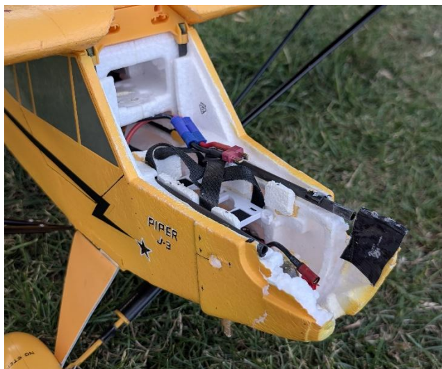
A close up of the ripped out motor and the lost hatch.
