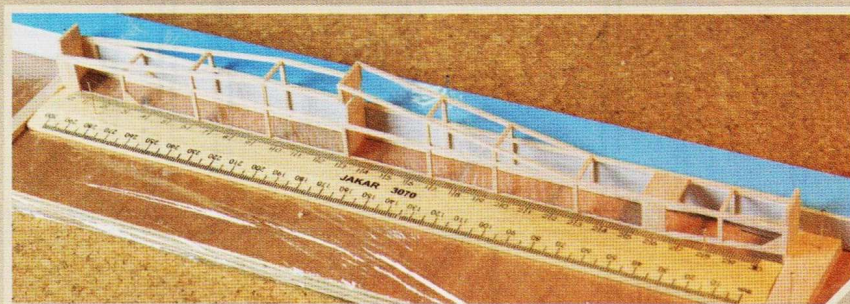
Temporary balsa formers help keep the fuselage sides spaced correctly while the cross pieces are added.
