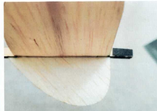
18) Glue one strip of sand paper to each side of the rear of the fuselage.
