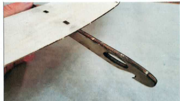
12) Repeat for the starboard side, again making sure that the plywood strengthener is perfectly aligned.
