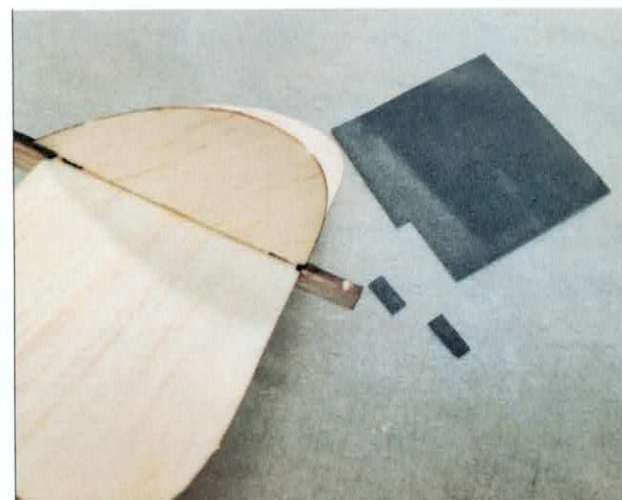
17) Cut two small strips of sand paper from the sheet provided.
