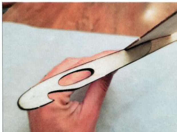
11) Glue the plywood strengthener to the port side of the fuselage, making sure that it aligns perfectly.
