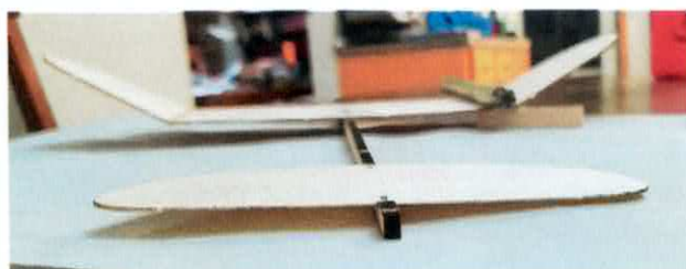
15) Make sure that the tailplane is well seated and flat.
