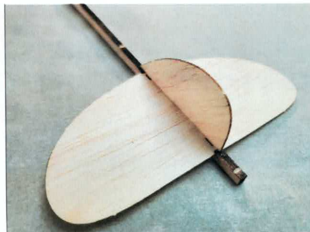
16) Glue the tail fin in place and make sure that it is perfectly vertical.
