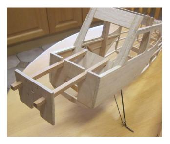
The undercarriage detail in the kit was an odd arrangement whereby the whole thing swung back restrained by rubber bands. A recipe for disaster, so we decided on a fixed, solidly built arrangement in the traditional style. There were no wheels with the kit, but fortunately I had a very suitable pair.
