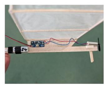
The timer is a BMK device bought from Mike Woodhouse at Free Flight Supplies. The motor came with a bigger prop, but this delivered too much power, so Roy found some smaller props and push fitted one onto the motor.
