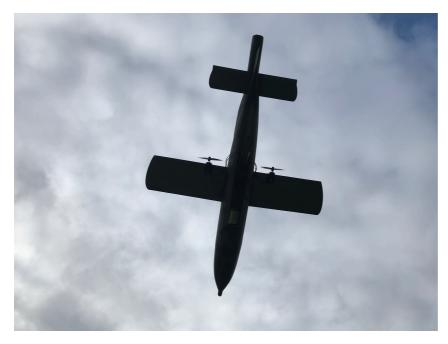
The FZG-76 looks fantastic in the air. thanks to the build quality by Chris, but because of the extra weight and high wing loading the motors were flat out screaming their little heads off. The landing speed is much higher than the JB-2 Loon, so even in long grass, the airframe could easily be damaged, as noted after inspection when I got home.
