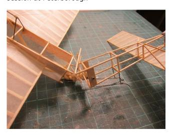
It slid down the wall and crunched into the ground where the energy in the rubber motor crushed the fragile fuselage
