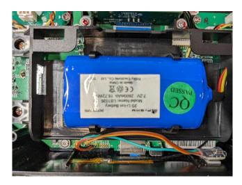
RC Video Reviews showed how to solder an ExpressLRS receiver into a transmitter to create a wireless buddy link, and I decided to do this with my old Horus X10S transmitter. The £10 receiver is a tiny 10mm square and can be seen in the bottom right corner of the photo. This now pairs up wirelessly with my new Boxer radio.
