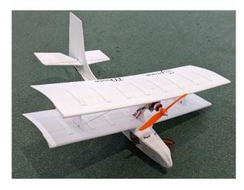
John Poleys 2mm Vector foam indoor RC biplane certainly has a moose like nose hence the name. It flew well and with the motor away from the nose is pretty crash resistant. It spans 450mm and weighs under 90g. There have been a lot of great new foam models recently!!
