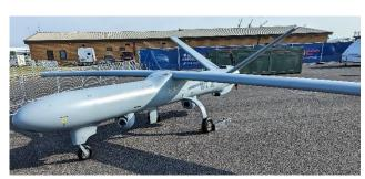
This the "Watchkeeper" RAF surveillance system. It uses a Wankel engine and can stay up for 14 hours cruising at 77 knots
