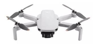
This is a drone. Typically the left stick for the throttle is spring centred in the middle. You push forward for up and when you let go the stick returns to the centre position and the drone stays where it is – usually with a combination of GPS and camera positioning. A drone requires less piloting skill and is essentially a flying platform for a camera.
