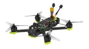
This is a quad. Its throttle works like a standard RC plane and you push forward for more power and pull back to reduce power. A quad flies faster and is aerobatic. If you take your hands off the sticks for more than a second or 2 it generally crashes, unlike the drone which just stays put till its battery gets too low when it lands itself.
