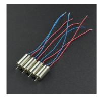
These coreless motors are just right for those who love to DIY drone models! Designed to be high-performance and easy to wire, the motor will work at a maximum of 3.7v. The compact size of 8x16/20mm can give out 50000 RPM. Combined with propellers, the motors are good choices for DIY projects like remote control aircraft too.
