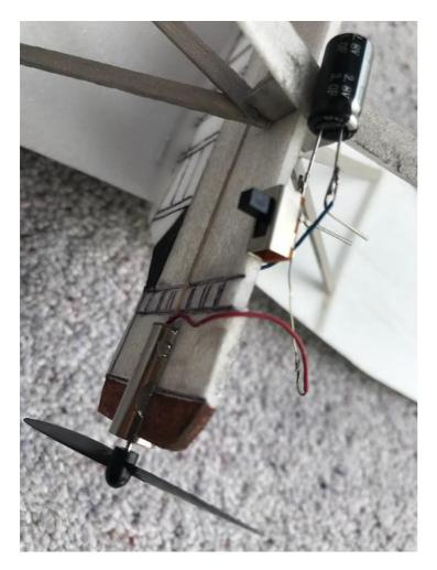
If you are flying indoors, build light, less than 16g AUW. and use the 2.7v 5Farad. Move up to 10Farad for bigger models or possibly a twin motor!
