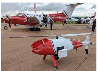
Spotted at Fairford is the Coastguards new S&R drone which they have now put into service. It's a Schiebel S-100 that weighs 200kg, flies at 55kts with a range of 200 miles
