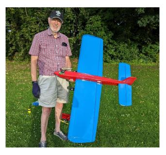
We last saw this on Chris Caruanas building board, but it had its first flights on a recent Friday evening. It's powered by an MDS 40 which previously powered an RC Piper Cub. It's now fitted with a non RC carburettor.
