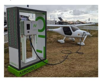
Spotted charging recently. This electric plane from Slovenia flies at 98kts for 50 minutes on one charge. The motor develops 57KW from its 2 x 345 Volt batteries that weigh 70Kg each. It takes about 2 hours to fast charge.
