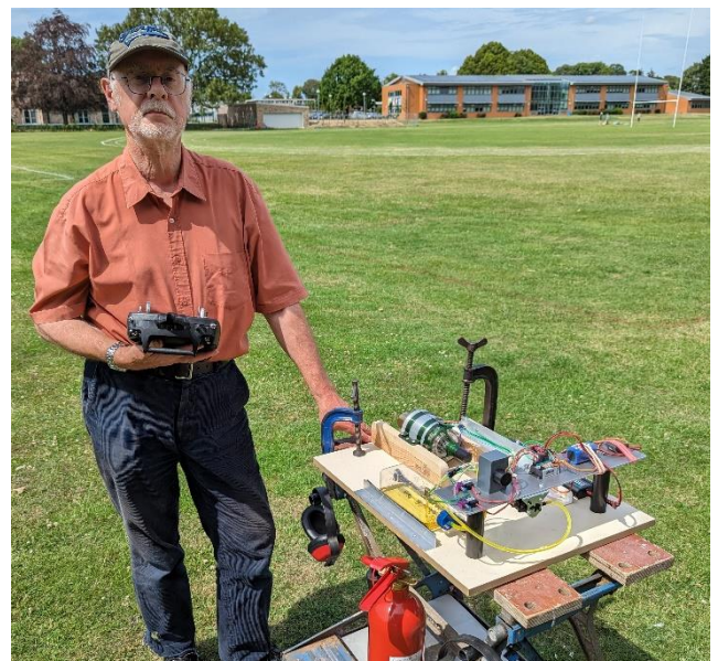
Tims Wren Turbine created a stir. It converts kerosene to noise and 18lbs thrust very well.
