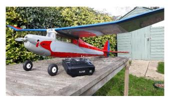
David Stophers winter build is a Valueplanes CloudWalker, a 'traditional' design now kitted in China. He knew it would be nose light (designed for IC originally), so added 2cm to nose length during build. That wasn't brave enough – it should have been about 4 or 5cm and needed about 100g in the nose even with an upgrade from 3S to 4S.
