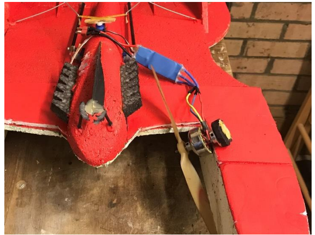
The motor detached from the mount after rescue from the tree
