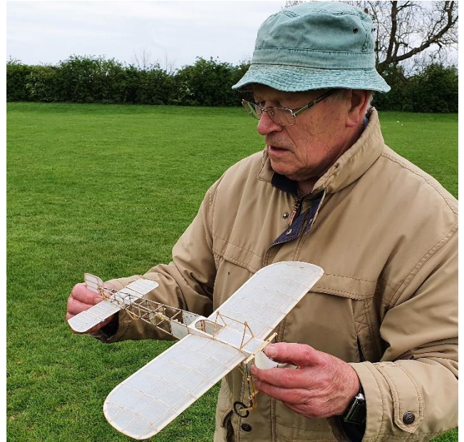
Gordons Bleriot is unusual in that it's a conversion of a radio model to free flight. Based on a Tony Ray kit it flew really well.
