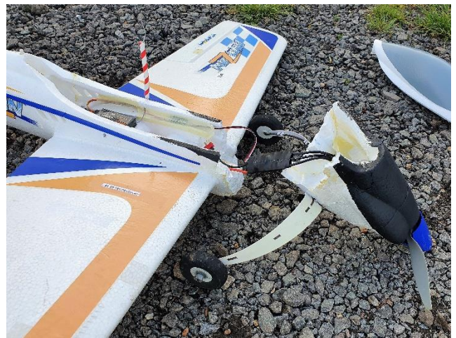
Alans Artizan after the canopy fell off during negative G, closely followed by the battery. Due to the wonder of UHU Por glue, this was flying again 2 days later!!
