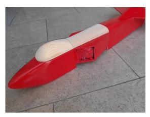
I don't know what the material is exactly, but as soon as you heat it up it goes back to a flat sheet reading for remoulding, and its exactly the right size for my moulder frame! The cockpit and hatch are fitted with two pins at the back, and a couple of magnets at the front. The hatch is hollow to cover the elevator servo (no rudder) and receiver.
