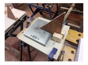
I found the 'kitchen scales adaptor' to be a bit unreliable, so invested in a 1Kg spring balance. The raw thrust is between 550g and 650g, very heavily dependent on the battery used. I did some experiments with inlet baffles and thrust pipes. The 'word on the street' (internet) is that the tail pipe should have slight nozzling to 85%-90% of the effective fan area (total area minus hub area), which proved about right.
