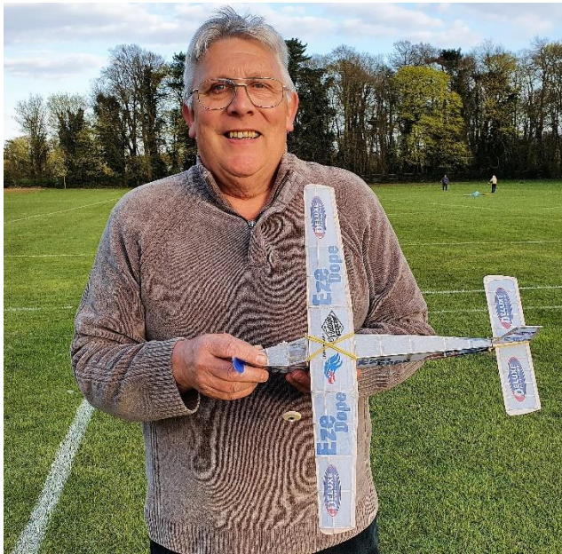
Stuart with his Sparrow Hawk by Vintage Model Company. Tissue covered using Deluxe Models Eze Dope which is a water based product that has no smell. Stuart guarantees that household friction caused by dope smells are a thing of the past!!
