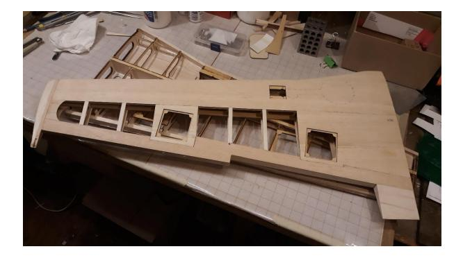
The only problem was with the second wing half, where the main spar had been hanging around for a few days and had somehow developed a curve. I didn't notice this until the wing was half built, and some emergency cutting and straightening was needed to remove (most of) this curve – a lesson there to check everything as you go.
