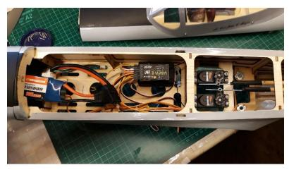
Time to look at making more space here by removing some of the tray to allow servo wiring to go up into the fuselage space. So we remove most of two panels, add ply strips reinforcement at edges to maintain structural stiffness ( the Engineer talking here), move the RX to the fuselage side, and hey presto.
