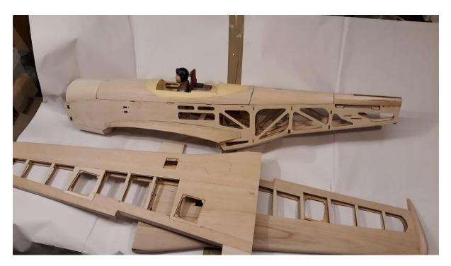
Lots of careful shaving and sanding, and we had two wings and a fuselage – the heavy lifting done.
