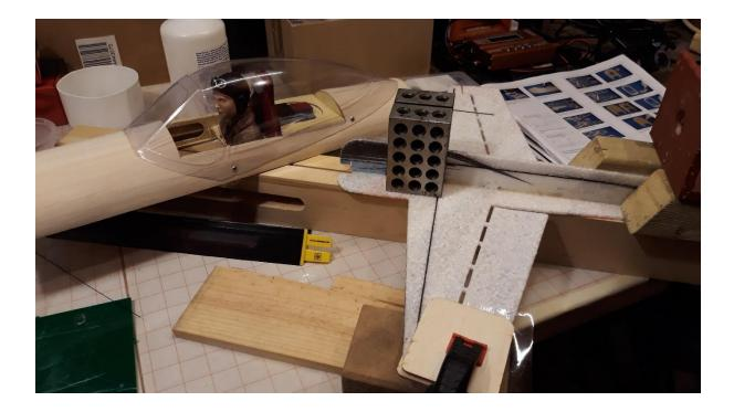
The photo also shows a little 400mm span indoor foam sheet plaything that I am concurrently materialising from a cheap Amazon/Ebay kit using, as the power train, various bits from previous disasters – who says that males can't multi task? My patented method of keeping the X-profile fuselage and everything else nice and square is shown next to the real work in hand. This technique wasn't entirely successful, but no doubt the little devil will still fly. Next up – the fuselage.
