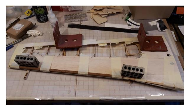
I added white glue along most edges after the upper skin was set for extra security. The finished wing was as stiff as a butcher's dead dog (after Boris Johnson, P.M.). Fixing the upper skin properly was critical, and a belt-and-braces approach was taken, involving pins, weights, masking tape and stiffeners to ensure straight edges.
