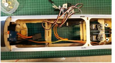
This modification also means the wing can be fixed before the servo leads are connected – much easier at the field. What a genius.
