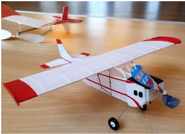
Clives new Lacey M10 sporting a prop made from a yoghurt pot – now that’s a good idea!!
