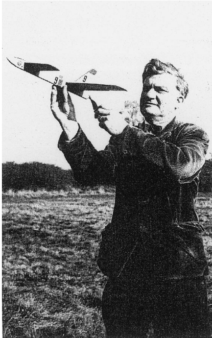
Author demonstrates launching technique. Plane must have adequate airspeed before release, no prop wash over surfaces.
