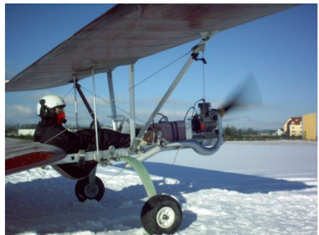
A Rotax 447 engine powered the prototype
