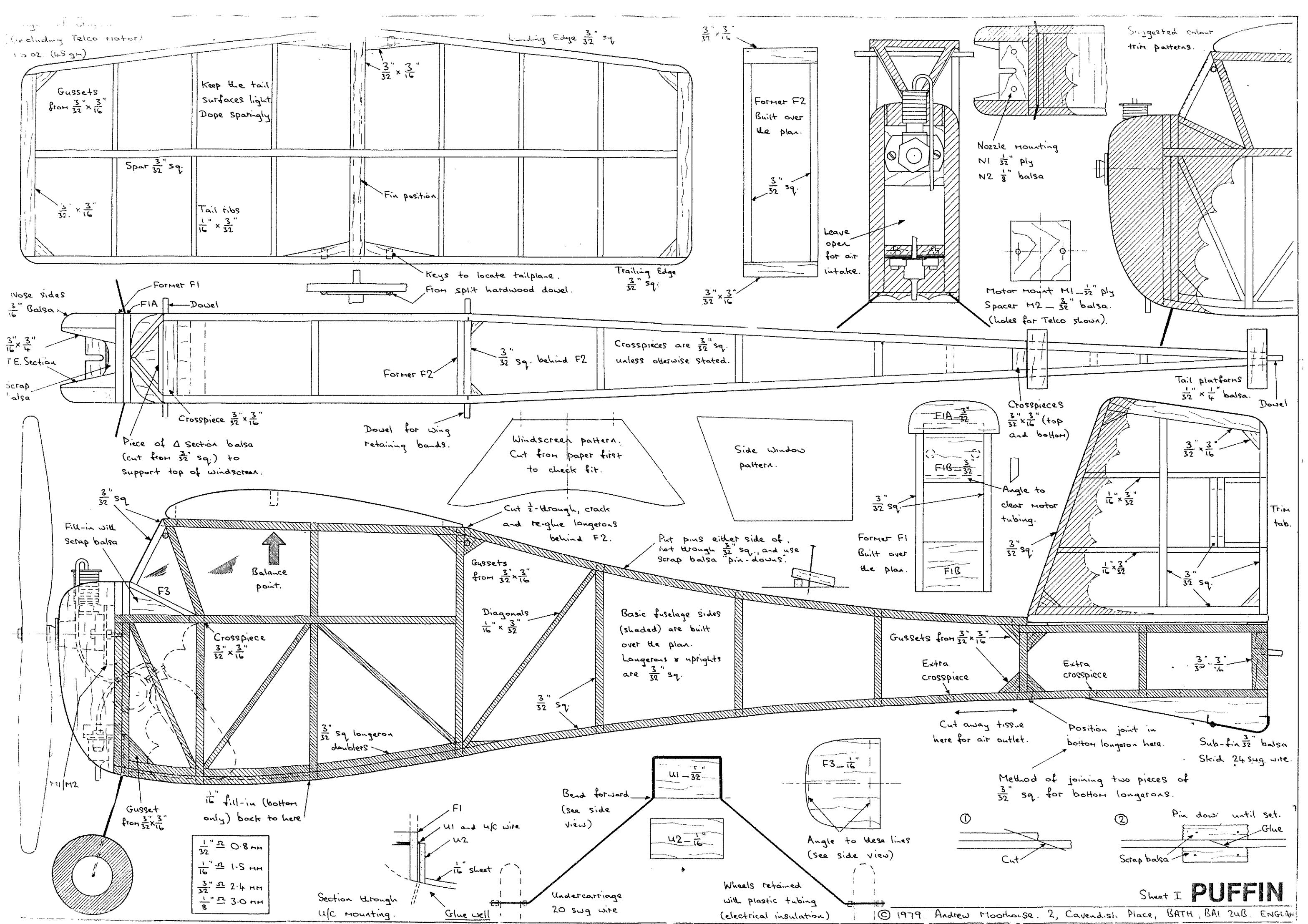
Before starting to build, study the plans and instructions carefully, and identify all the pre-cut and printed parts, and the different sizes of strip balsa. Choose strips of suitable grade for each component, e.g. medium-hard or hard  $\frac{3}{32}$ " sq. for the fuselage longerons, lighter wood for the tail surfaces, and so on.
