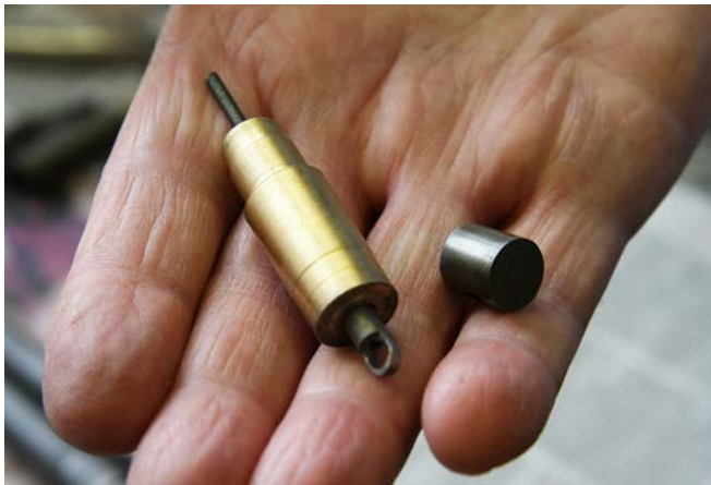
jig for holding the piston while lapping
