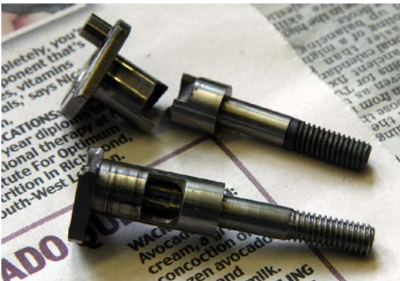
prop shaft, below, made to replace the broken one above from a CS tiger cub . . . worked well until it too had a mishap
