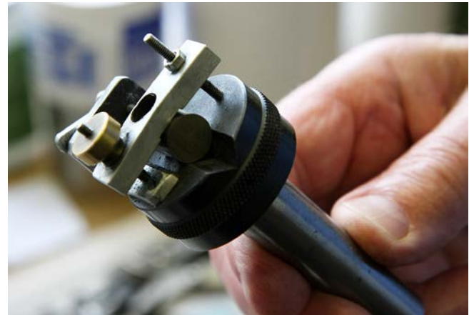
piston in jig and ready for drilling to take the gudgeon pin
