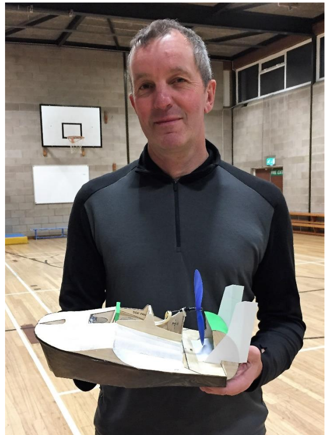
It definitely qualifies as an aircraft. This is Clive Holgates rubber powered hovercraft. It's yet to be finished but was having test flights in the gym. The green scoop at the back picks up the airflow from the prop to form the cushion on which the craft rides.
