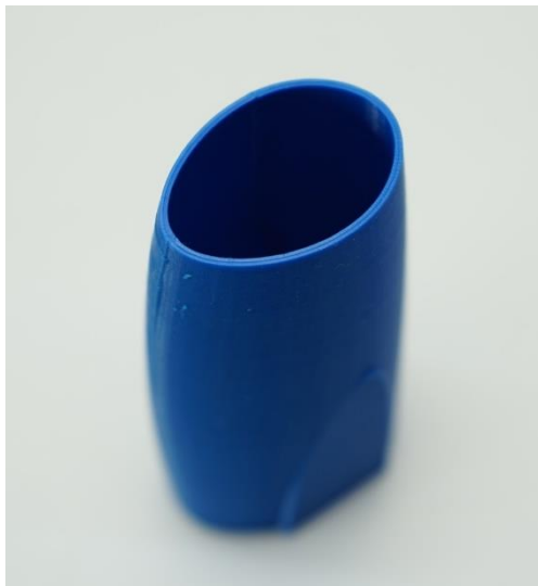
Fuselage section after printing
