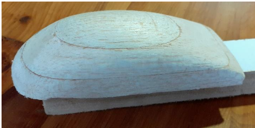
Initially create a balsa "plug" for the canopy
