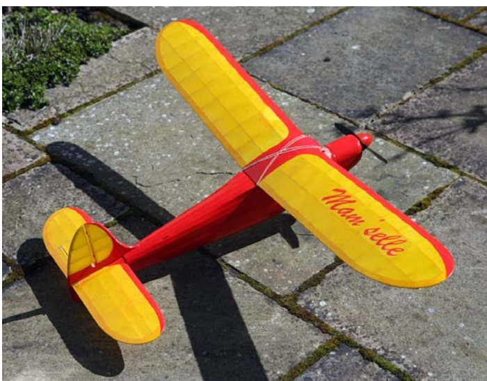
covered in Polyspan and combining old with new
