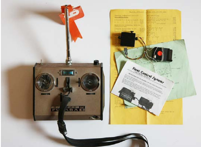
Tony's modified Tx, servo and Rx
