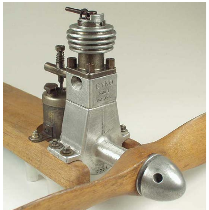
The 2cc Swiss Dyno of 1940 was the first commercial model aero diesel engine
