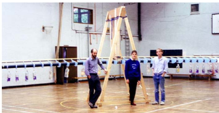
load testing the spar: me, pilot and engine Nick Weston and Mark McIntyre
