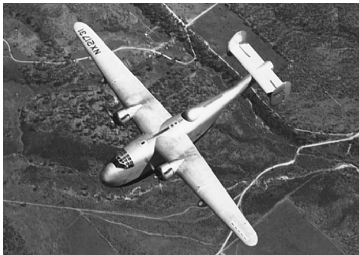
The Davis wing in use on the XP4Y Corregidor vindicating the design
