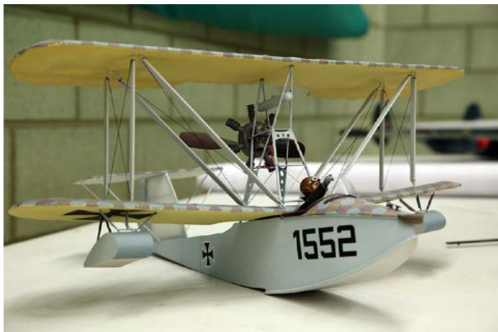
Hansa-Brandenburg W.20 designed to be stored and launched from a submarine
