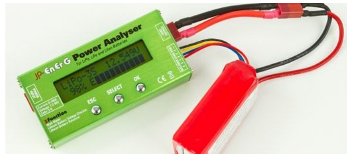
The display reads: LiPo 3S 12.549V 98% capacity
