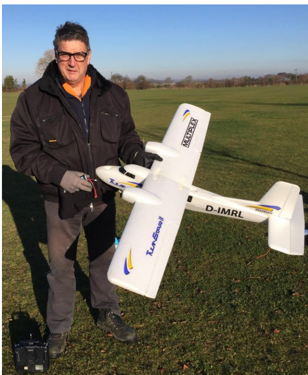
Steve Mynotts passengers would not enjoy the ride. This Twinstar does amazing low level aerobatics and has also had the odd repair – luckily he got it free and has given it a good home. It runs well on old fashioned brushed motors and 2S Lipos rather than the old Nicads the kit was designed for.
