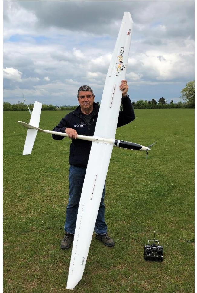
Steve with his Multiplex Kranich (the Crane in German). This is a model that dates from the last millennium but still flies beautifully. At 2.9m wingspan and weighing a hefty 3Kg+ it takes a positive launch to get it going.
