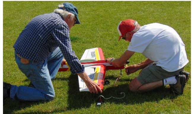
Robin Soanes returning the favour for John Ash who is starting the SC52 engine in his own design Cruiser model. This one is the 6th development stage of John's own design.
