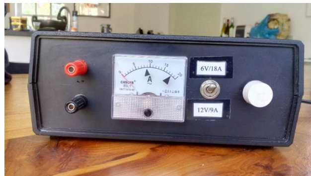
Front panel layout. Note the maximum current markers on the meter
