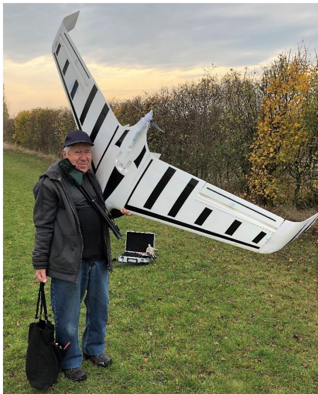
Norman manages to carry his huge 2m wingspan Optera flying wing. This is an amazing model that Norman can self launch due to the inbuilt stabilisation system.
