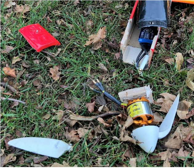
The damage caused by the vibration shook the nose of the model to pieces!!
