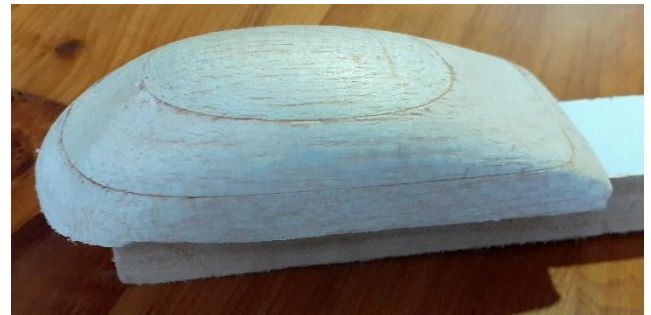
Initially create a balsa "plug" for the canopy
