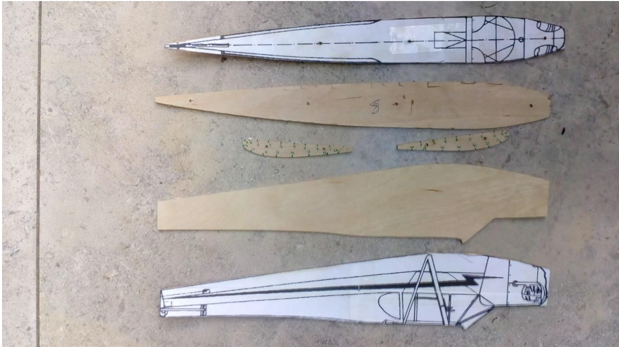
Templates in 1mm ply for a DIY Foamie
