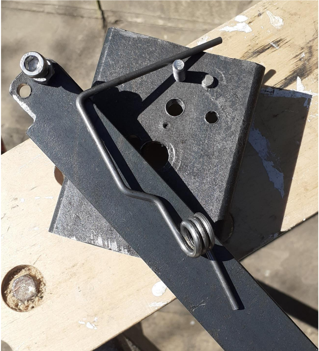
'Precision' set up with mandrel and bit closer together (at the other end of the lever) to do fine bending.
