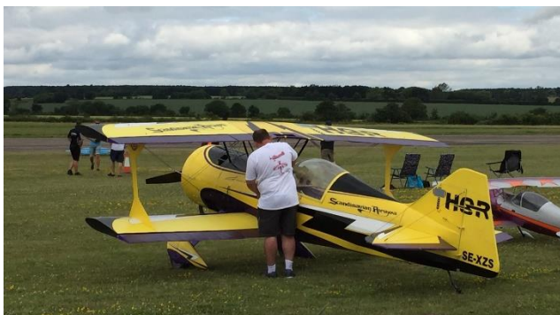
Pitts "Thor". This 87% scale model has a 650cc engine and a 68" 3 bladed prop. Almost makes you want to jump in it for a flight – but check the pilot out first.....
