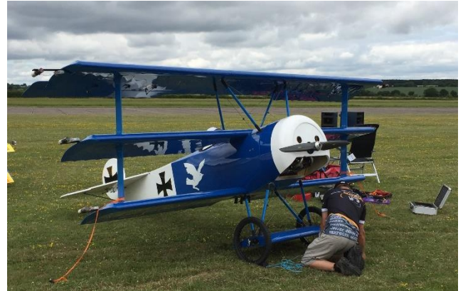
Fokker DR1. This is 65% scale with a span of 4.8m. It took off in about 10 feet and has a home brew 550cc engine. You can actually buy this model as an ARTF kit!!
