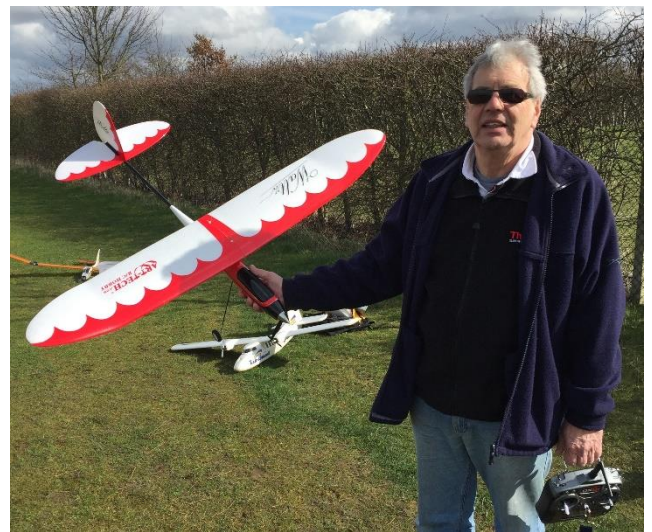
A nice little 46" span retro styled 3 channel model with a brushless motor and powered by a 2 cell 1000MAh Lipo. This one is Mick Flacks which had its maiden flights at Cottenham on 7 th March – the first time we had been out flying there for a few weeks. You can also see Steves Twinstar lurking in the background.
